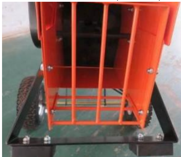
Pic.5 Fence netting installation
